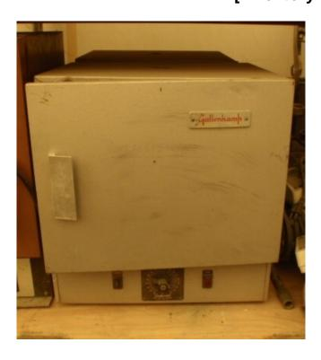
Gallenkamp Lab Ovens. Inside chamber 15 in. x 12 in. x 11 in. 110 volts, 4.6 amps. One tray and control dia.
