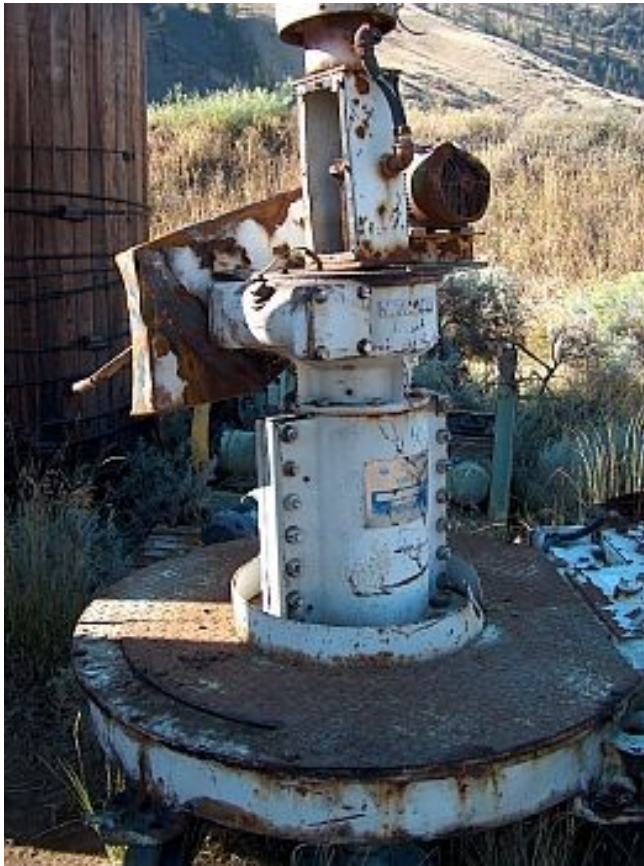
Eimco 48 inch clarifier/agitator head. Type B. Model# 110E2278. Unit supplied refurbished.
