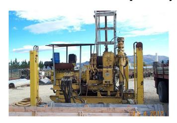
Edeco Stratadrill 80 Diamond Core Drill with HQ Chuck, 6 Cylinder Deutz Drive, Located in New Zealand
