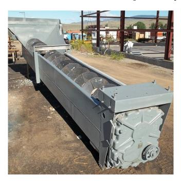
Eagle 30 inch dia. X 25 ft long Sand Screw. Supplied with complete set of new wear shoes.
