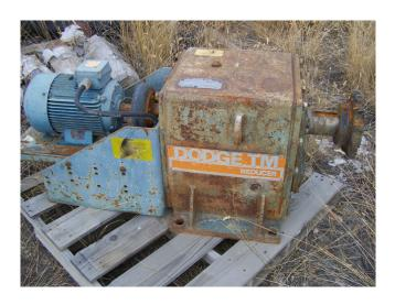
Dodge Inline Gear Reducer, Model TR 800 194.6 to 1 Ratio, Comes with 5 HP 1155 RPM Motor.
