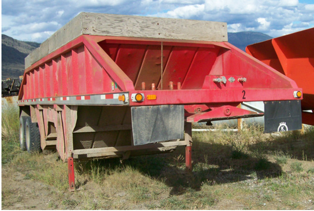
Decap Bell Dump Trailer. 8 Ft.W x 32 Ft.L x 8 Ft.H. Air Operated Clam Gates.
