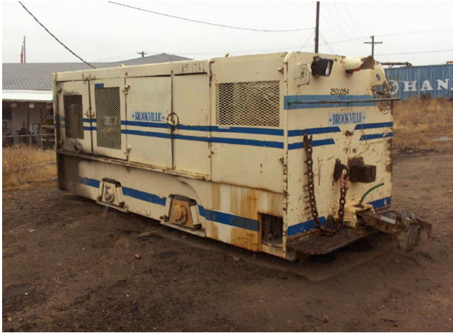
Brookville 15 Ton Locomotive. 36 in. Gauge. Diesel Driven.
