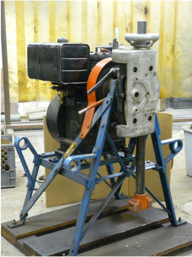
Boyles X-Ray Diamond Drill. Gas Motor Drive.
