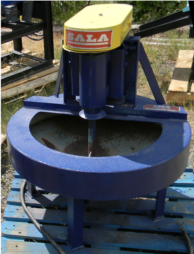
Bomba de Tanque Vertical Sala SPV 181
