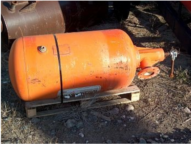
Bin and hopper Air cannon. 24 in. dia. x 48 in.
