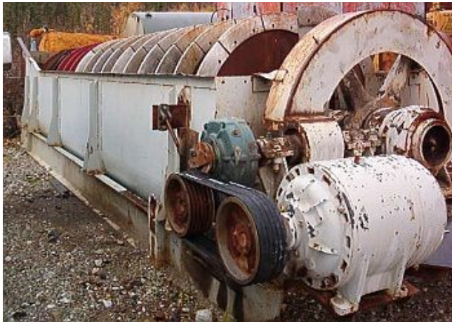
60 in. Sandscrew Classifier. c/w Mixed Urathane & Steel Wear Plates.
