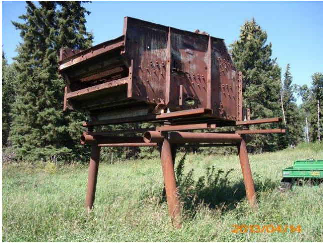
6 ft. x 10 ft. 2 Deck Allis Chalmers Vibrating Stepped Screen.
