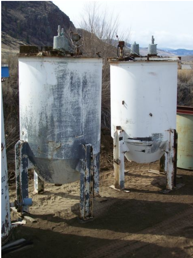
6 ft. dia. x 10 ft. Steel Conical Pump box with 3 ft. Legs. Dual 8 in. Discharges.
