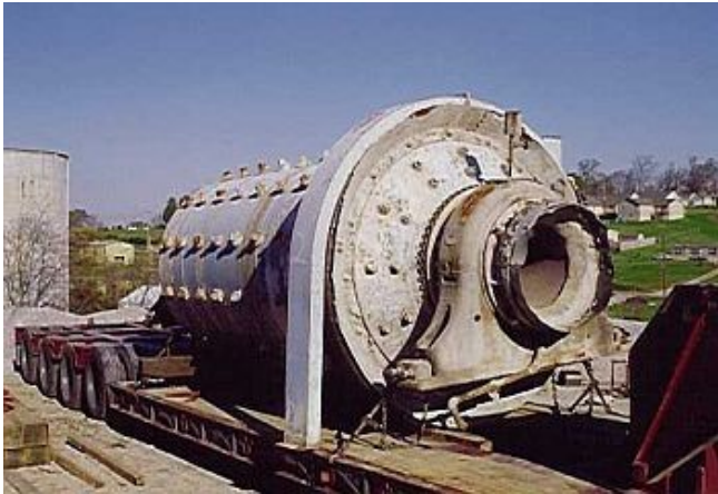
6 foot x 12 foot Hardinge Rod Mill, c/w motor reducer drive
