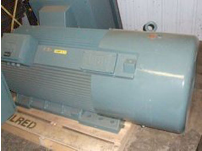
500 HP Weg Electric Motor, TEFC, 4160 Volt, 1782 RPM, 5011 Frame
