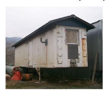
40-foot generator/parts van. Tandem axle with 5th wheel pin and landing gear. Air intake louvres at both ends.
