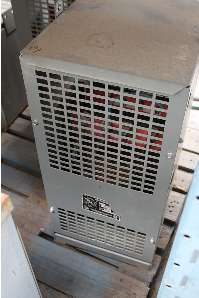
37.5 KVA 480 - 120/240 Single Phase Indoor Dry Marcus Transformer
