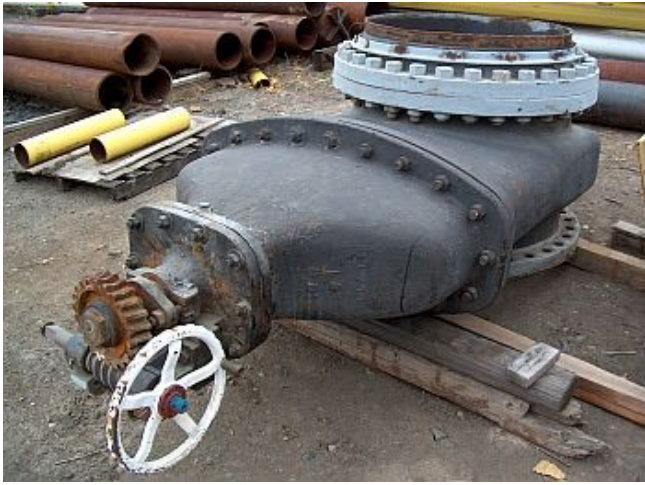
36 inch Glenfeild gear trim operated gate valve
