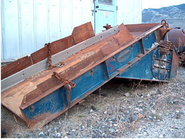
36 in. Wide x 8 ft Long Forano Vibrating Feeder, 3 HP, 575 Volt
