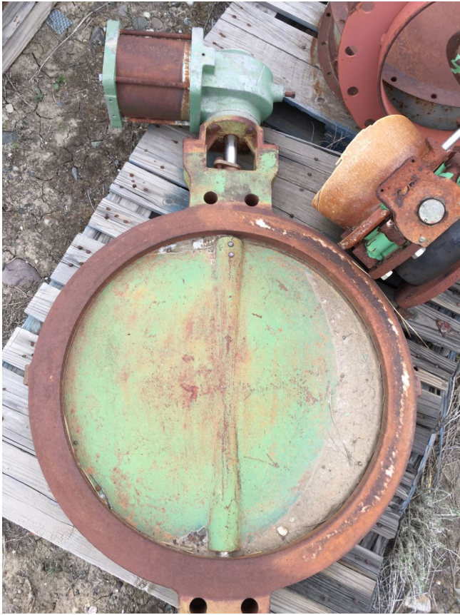
30 in. Air Operated Butterfly Valve.
