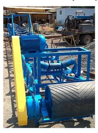
24 inch x 84 foot truss conveyor. Comes with shaft mount reducer and electric drive motor. SUPPLIED REFURBISHED
