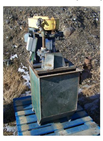
1.5 in. Galigher Sump Pump. Model: 15-SR-2100-24. Belt Driven 5 hp 1750 RPM Electric Motor. Mounted on Caster wheels.
