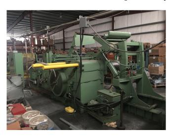
Horsepower: 40 HPCapacity: 10,000 lbs.Slitter: 36 in. Wide
