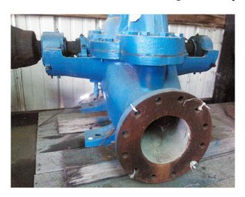
Size: 8 in. x 5 in.Model: 5LN-22.22 inch impeller.
