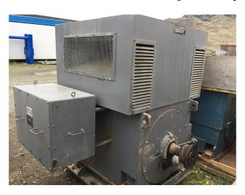
HP: 700RPM: 712Volts: 575Frame: 4509Type: HSAmp: 7343 Phase60 Hz
