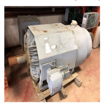
HP: 400Voltage: 575Frame: 5806B1800 RPMBall Bearing
