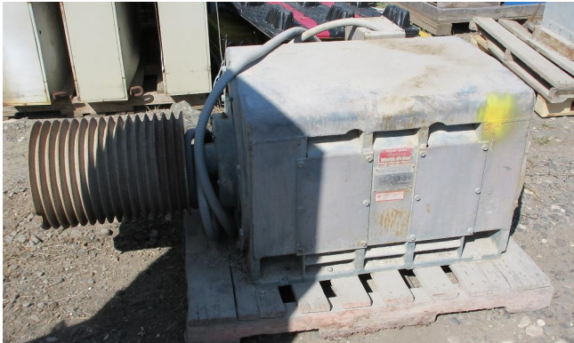
Westinghouse 250HP LAC Induction Motor
