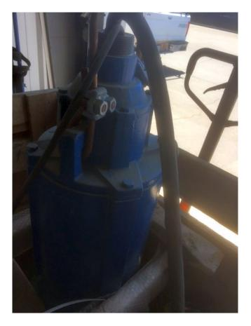
Make: Torque-Flow-Pump - vertical submersible Model: Model E - LRS Year: 2014
