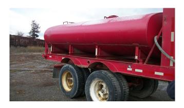
Water Tank Trailer. 2500 Gallon Capacity. Honda Pump & All Hoses.
