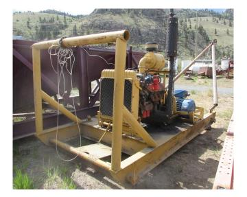
Warman 8/6 EEXU Diesel Driven Slurry Pump
