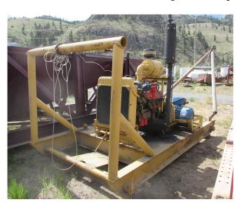
Warman 8/6 EEXU Diesel Driven Slurry Pump
