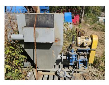
Warman 1½ x 1 AH Slurry Pump with Pump Box
