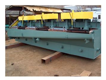
We will buy or sell your new or used flotation cells used for the recovery and upgrading of sulfide ores. We will buy and sell various brands and sizes of floatation cells including Denver, Hazen Quinn, Wemco, Outokumpu, and OK Floation Cells
