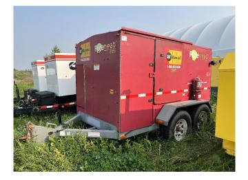
Wacker Neuson Pureheat Hydronic Portable Air Heater
