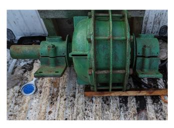
W.W. Gibson Combination Elliptic Roll and Ball Mill
