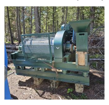
W.W. Gibson 2ft Dia. x 4ft Ball Mill
