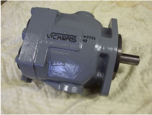
Vickers PVB 15 Hydraulic pump.
