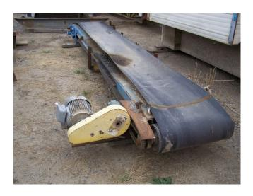
Used Square Tubing Conveyor. 24 in. x 15 ft. Long. 5 HP Motor through Radicon Reducer.
