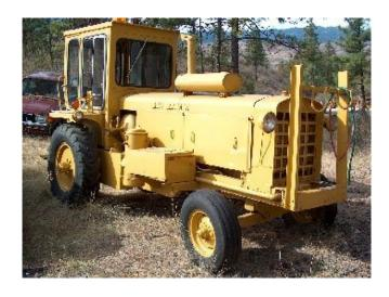
Used Schramm 300 CFM Diesel Compressor. Tractor chassis with GM 471 diesel drive.
