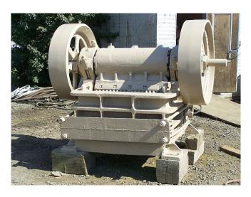
Used Roller Bearing Jaw Crusher. 9 in. x 36 in. 50 HP Electric Motor.
