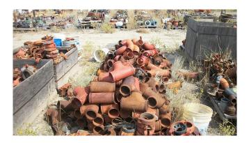
Used Pipe Fittings. 4 in. to 6 in. Grooved Fittings, Clamps, Elbows, Ts, Ys & Reducers
