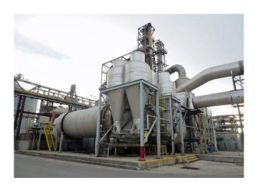
Used ICM Stainless Steel Rotary Dryers. 13.5 ft. dia. x 40 ft. Long. Model: 40136L. Eclipse 22V Burner with 400 HP Fan. Each System has 4 - 8 ft. dia. Cyclones.
