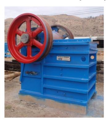
Used Hewitt Robins King Jaw Crusher. 30 in. x 48 in. 150 HP Electric Motor.
