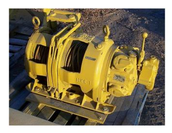
Used Gardner Denver (Slusher) Hoist. Model: HKE. Double Drum - Air Operated.
