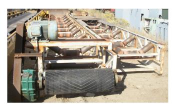
Used Channel Conveyor. 36 in. x 80 ft. Long. 15 HP Motor.
