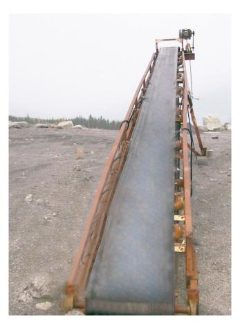
Used Channel Conveyor. 24 in. x 40 ft. Long. Comes with Support Legs.
