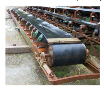
Used Channel Conveyor. 24 in. x 35 ft. Long. c/w Steel Head & Tail Pulley.
