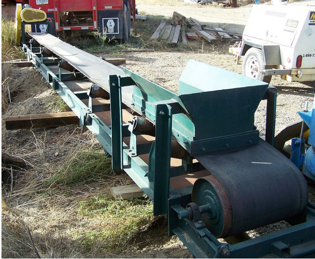
Used Channel Conveyor. 18 in. x 30 ft. Long. 2 HP Single Phase Electric Motor.
