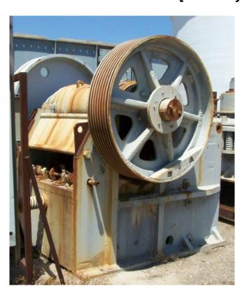
Used Cedarapids Jaw Crusher. 25 in. x 40 in. New Jaw Plates & Bearings.
