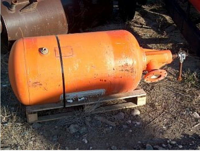
Used Bin and hopper Air cannon. 24 in. dia. x 48 in.
