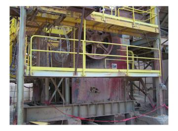
Used Austin Western (BLH) Jaw Crusher. 42 in. x 48 in. Roller Bearing Style.
